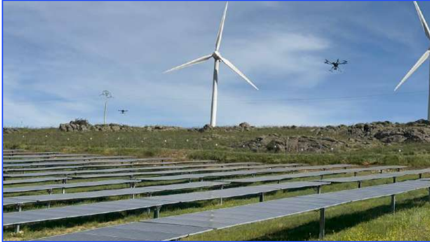
Simultaneous inspection with 2 autonomous UAVs
