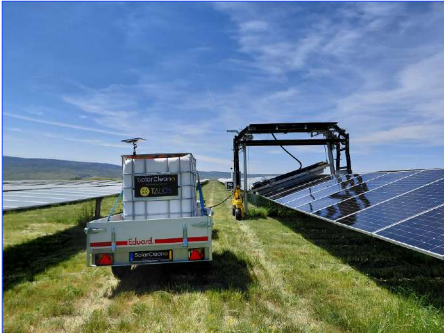
Integrated cleaner + water carrier system
