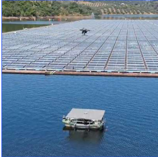
Simultaneous inspection with UAV and USV platform
